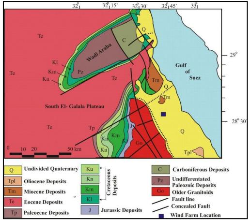
Figure 8-11: Regional Geologic Map of the Area (Modified from the Egyptian Geological Survey and Mining Authority, 1981)
