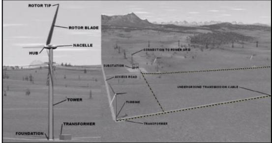
Figure 3-5: (a) Typical Structural Components of a Wind Turbine, (b) Typical Components of a Wind Farm (Source: EHS Guidelines for Wind Energy, IFC)
